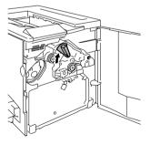
2 Grasp the release lever on the OPC drum cartridge, and then pull the cartridge straight out about 6 inches (152 mm).
